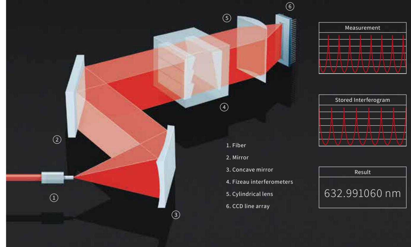
The light is coupled into the device via a fiber and then collimated by a mirror, before entering the solid-state Fizeau-interferometers. The interference pattern is imaged by a cylindrical lens onto CCD photodiode arrays. This recorded pattern is transferred to your computer via a high-speed USB connection which allows data acquisition rates of up to 50 kHz.
